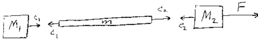
$$c_1 = M_1 a \quad c_2 - c_1 = m a \quad F - c_2 = M_2 a$$
