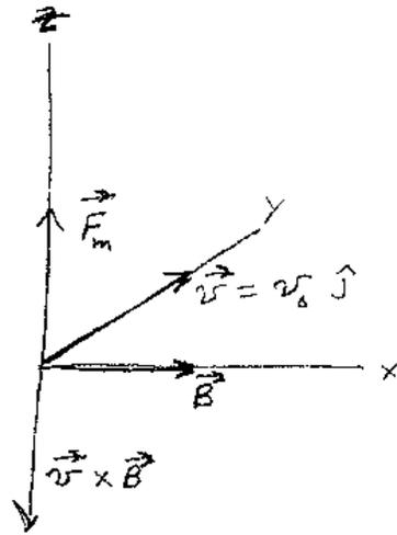
$$\begin{aligned} \vec{F}_m &= -e(v_0 \hat{j} \times B_0 \hat{i}) \\ &= e v_0 B_0 (\hat{i} \times \hat{j}) \\ &= e v_0 B_0 \hat{k} \end{aligned}$$
