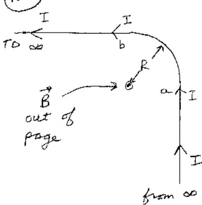
$$\vec{B}_{\text{NET}} = \vec{B}_{\text{from } \infty \text{ to } a} + \vec{B}_{a \rightarrow b} + \vec{B}_{b \text{ to } \infty}$$
