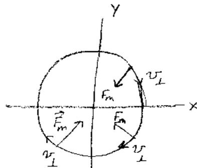
the charge of the electron is negative, this means that  $\vec{v} \times \vec{B}$  for the electron must point towards the lower right corner of the diagram. Since  $\vec{v}$  is towards the upper right corner of the diagram, the direction of  $\vec{B}$  must be **out of the page**.
