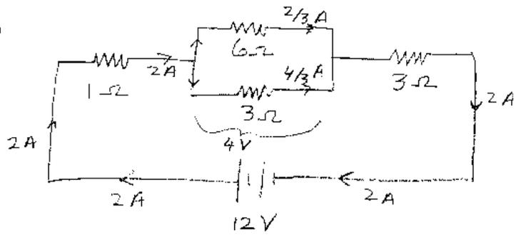
$$\frac{1}{R_{36}} = \frac{1}{3} + \frac{1}{6} = \frac{2}{6} \quad R_{36} = 3\Omega$$
