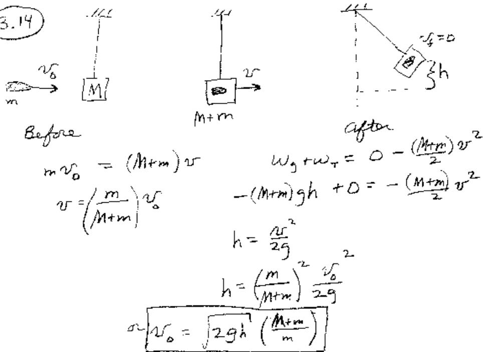
The work  $W_T$  done by the tension in the string is zero, since the direction of this force is perpendicular to the direction of the block's velocity. The work  $W_g$  done by gravity is negative since the block moves upward in the opposite direction of the gravitational force. Substituting for  $v$  in the second equation gives
