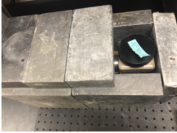
Fig. 4. Soil measurement setup. When the spectrum is collected, bricks are added to cover up the sample and detector. During collection, the sample and detector are completely shielded by 5 cm of lead.
