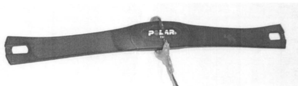
Fig. 2. Coil of wire that is placed around the heart rate monitor to pick up the transmitted signal. With 80 turns of wire, the resulting signal has a peak-to-peak voltage of 0.8 V.
