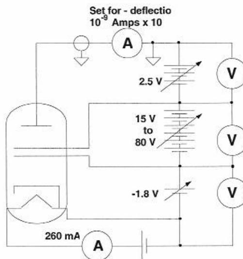
As the main power supply voltage increases minima are observed in the anode current (measured in the top ammeter above). With each minimum a new, sharp layer of glowing neon atoms are observed. Plot a graph of anode current versus applied voltage. Measure the average difference in the voltage between current minima (or between current maxima) to obtain the quantum of energy that neon atoms can absorb. Compare it with the energy emitted by the neon as light. Is it the same? Should it be?
