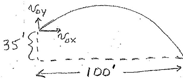
$$v_{0x} = \frac{100 \text{ ft}}{5 \text{ sec}} = 20 \text{ ft/s}$$
